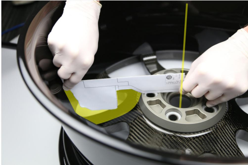
Allow 3mm in all directions from the caliper to the wheel. Note: the imagery and highlighted areas is meant to be an approximation to help illustrate the tutorial.
