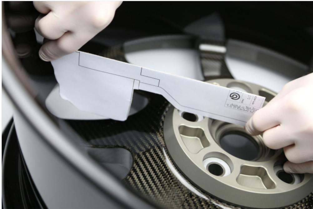
Place the cut-out inside the wheel well. If the cut-out is too flimsy, you may need to adhere it to a piece of cardboard to help with getting a proper gauge on your brake to wheel clearance.
